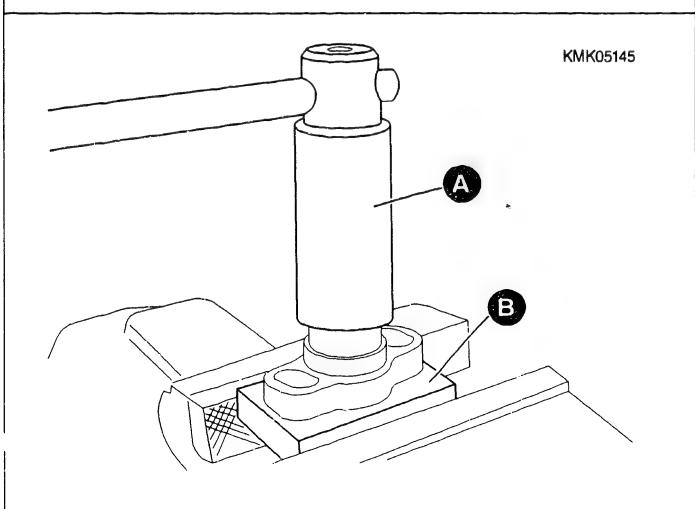
DISASSEMBLY OF BARREL-AND-VALVE ELEMENT
